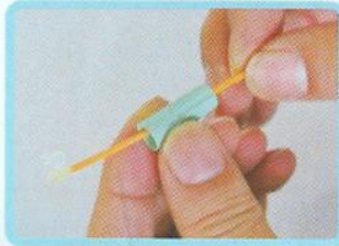
Put the cable into the boot
