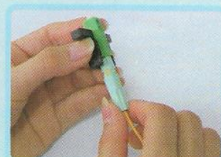
Unlock the boot, Put out the fiber
