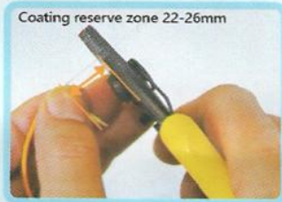
Strip the Φ 0.25 mm fiber coating layer
