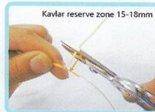
Shear the kevlar line
